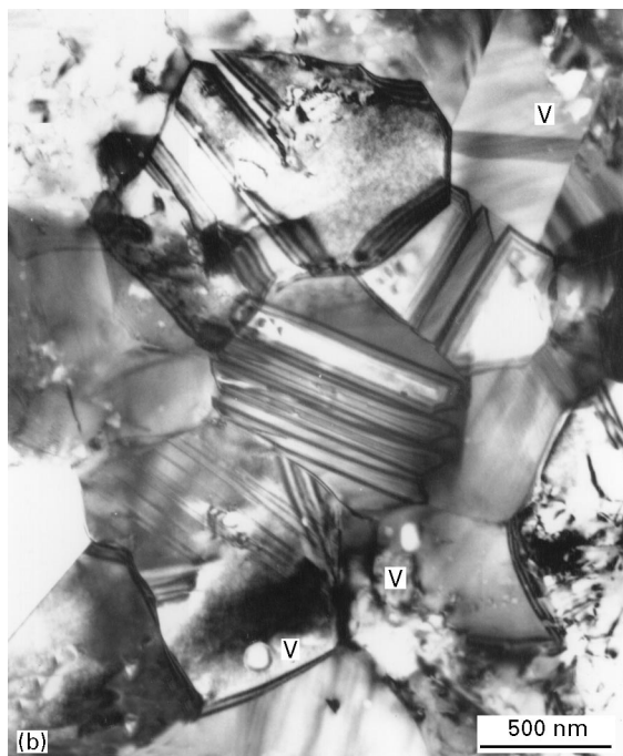
Figure 4 Bright-field planar view transmission electron micrographs of (a) copper-rich and (b) indium-rich samples, prepared by the selenization of metallic precursors.
